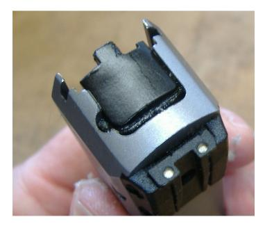
Now you can use a normal-sized screwdriver (and/or fingers) to slide the back cap the rest of the way off.
