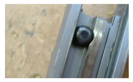
Here's a shot of the upper part of the firing-pin block with the extractor removed. The extractor has a "shelf" that slides into the recess (visible near the bottom of the slot) to keep firing pin block from falling out.
