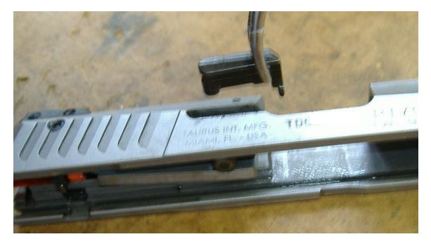
Here's what the extractor look like from above. Note the small notch on the left side. A spring-loaded wedge engages that notch and that's all that holds the extractor in place. The piston, discussed above, is what pushes against the other end of the spring that presses against the wedge.
