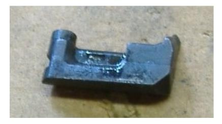
Reassembly is pretty-much the reverse. The extractor just snaps back in but make sure the wedge correctly engages the notch (the wedge can rotate to be 90 degrees from the notch so it won't engage). The firing-pin assembly just slides back in and it can only go one way.
