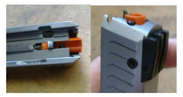
Here is the firing pin assembly out of the gun. The big spring (between the orange sleeve and the head of the firing pin) propels the striker into the primer; that same spring locks the orange sleeve into the detent in the plastic end cap we just removed. The "cutout" just behind the pointy end is part of the firing-pin block system and the hole at the top of the orange plastic sleeve is for the safety key-lock system.
