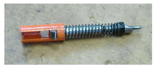
Here is <u>one important caution before removing the extractor</u>. The extractor holds the firing pin block in place. So be careful not to loose that part when the extractor is out. The firing-pin block is under light spring pressure and will easily fall out if you aren't careful. Here in the firing pin block on the underside of the slide.
