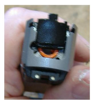
Before continuing, note the inside of the back cap. There is a circular recess that locks against the orange sleeve under spring tension. Also the cap is reinforced with a piece of metal.
