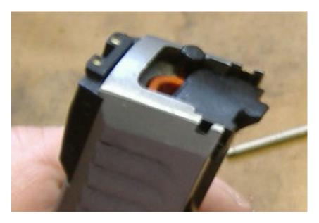
Then use a tool to hold the extractor piston into the slide while you push the cap the rest of the way.
